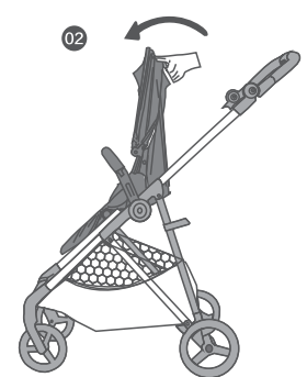
Figure 14-2: Folding the stroller (step 2) 2. Push seat forward.
