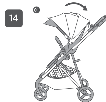
Figure 14-1: Folding the stroller (step 1) 1. Retract canopy.
